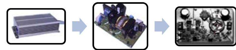
Figure 1 1) Iron core transformer, eff~85% 2) Isolated Switch Mode Converter, eff~92% 3) Piezotransformer-based converter, eff~98%
